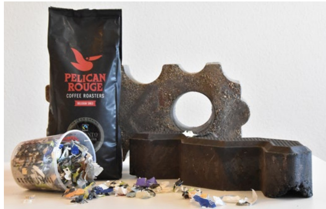
Road vibratory silent blocks made from coffee plastic bags.
